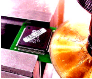
Fig. 9: QFP removal procedure
