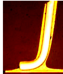
Fig. 12: SnPb lead finish on Sn/37Pb solder paste with 8 hour steam aging
