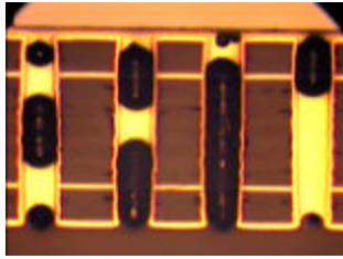
Figure 6: Cross-section of Unfilled Thermal Vias [5]
