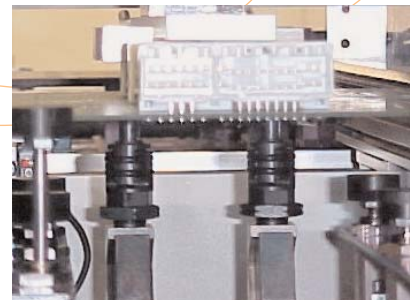
Dual, underside screw driving on connectors
