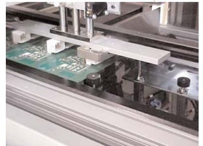
Secured connectors ready for screw driving
