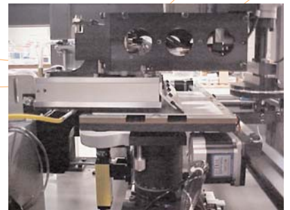
Post-placement label squeegee (side view)
